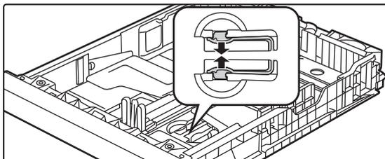
To load 8-1/2" x 14" size paper in tray 1 or tray 2, release the knob and stretch the tray to the point where it locks. After the tray is extended, move plate A to the front of the tray.
