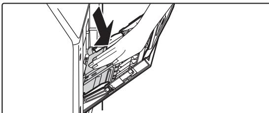
Push the center of the pressure plate down until it locks into place.
