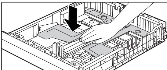
When using the tray, push the center of the pressure plate down until it locks into place.
