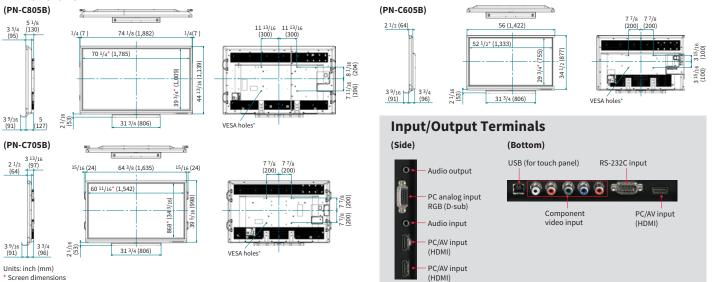
Screen dimensions \* To use the VESA-standard mounting bracket, use M6 screws that are 8 to 10 mm plus the thickness of the bracket
