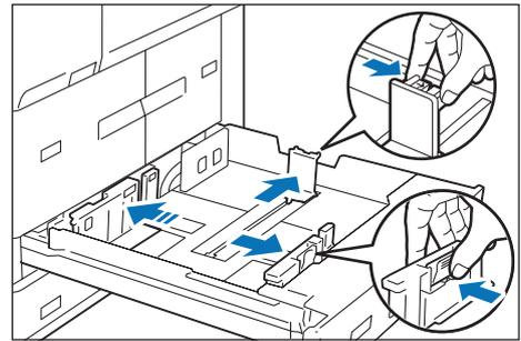
There are two guide clips on the tray 1 and 2 and one guide clip on the tray 3 and 4.
