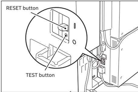
2. Check that the RESET button is turned OFF and in the "O" state.
