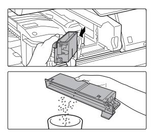
Grasp the punch waste box handle, gently pull out the box, and discard the punch waste.
