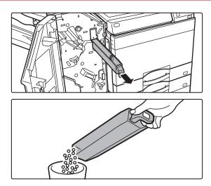
Pull out the punch waste box and discard the punch waste.
