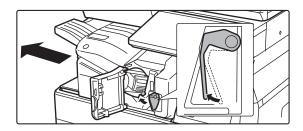
While pressing the lever over to the left, slide the finisher to the left until it stops.
