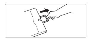
Pull out the extension guide of the bypass tray.
