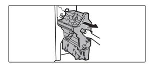
Pull the lever and withdraw the staple unit.
