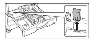
Remove the control plate auxiliary block.
