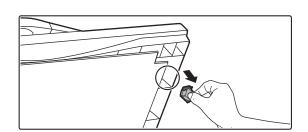
Open the automatic document feeder and remove the glass cleaner.
