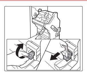
Lower the staple case release lever and remove the staple case.
