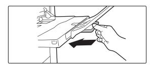
Replace the extension guide of the bypass tray.
