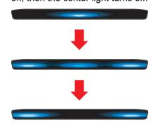
If the lighting state and the blinking state overlap, the blinking state takes priority.
