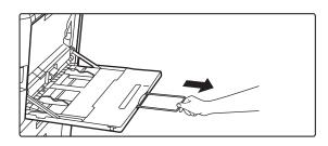
When loading paper larger than 8-1/2" x 11"R or A4R, pull out the extension guide.
