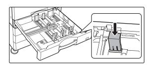
Attach the control plate auxiliary block that was removed in step 1.
