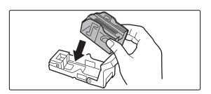
Insert a new staple cartridge into the staple case.
