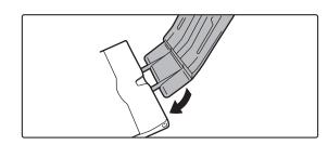
Attach the long paper feeding tray onto the extension guide of the bypass tray.
