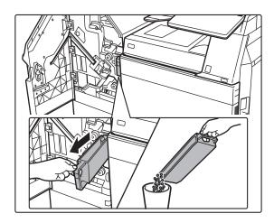
Pull out the punch waste box and discard the punch waste.
