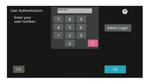
• If "A Warning when Login Fails" is enabled in the system settings, the operation panel will be locked for five minutes if an incorrect user number is entered three times in a row.
