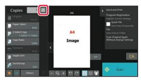
In normal mode, you can tap [File] or [Quick File] on the action panel before starting the copy job to save the scanned original as a file.
