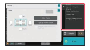
The functions displayed on the action panel vary depending on the mode or the functions that have been configured. If too many functions have been configured to be displayed on the action panel, you can slide the panel vertically or tap and to view all.
