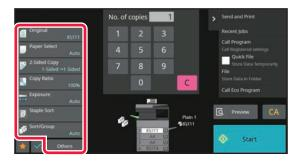
SELECTING THE ORIENTATION AND SIZE OF THE ORIGINAL (page 3-27) SELECTING THE PAPER TRAY FOR COPYING (page 3-13) AUTOMATIC 2-SIDED COPYING (page 3-14) ENLARGING/REDUCING THE LENGTH AND WIDTH SEPARATELY (page 3-24) AUTOMATIC ADJUSTMENT OF EXPOSURE AND ORIGINAL TYPE (page 3-18) OUTPUT (page 3-35) OTHER FUNCTIONS (page 3-53)
