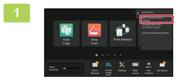
Open the action panel on the home screen, and tap [MFP Display Pattern Setting].
