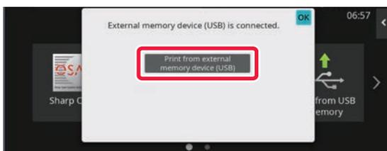
When a screen for selecting the action appears, tap **[Print from external memory device (USB)]**.
