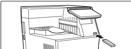
When you tap **[Select File from USB Memory to Print]**, connect the **USB memory device to the machine.**
