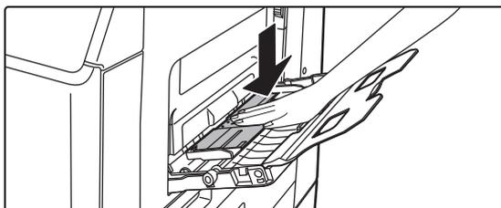
Push the center of the pressure plate down until it locks into place.
