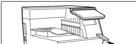
**Remove the USB memory device from the machine.**
