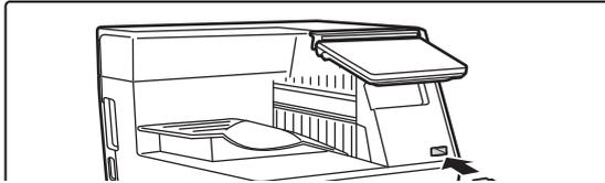
**Connect the USB memory device to the machine.**
