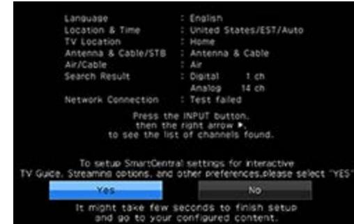
When no channel is received after "Antenna & Cable" was selected in step 6 and a search was carried out.
