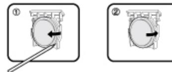
4 Align the battery holder with the battery slot on the 3D glasses and slide it back into place.
