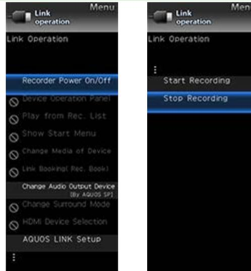
The Link Operation Menu allows you to make adjustments during operation of AQUOS LINK-compatible equipment.
