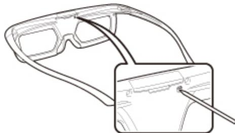
2 While pressing in on the lock, place your fingertip in the groove and pull out the battery holder.
