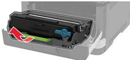
**3** Twist the blue latch, and then remove the used toner cartridge from the imaging unit.
