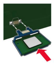
**Note:** The entire length of the connector on the card must touch and be flush against the controller board.
