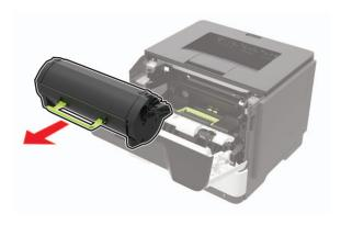
**3** Remove the used imaging unit.
