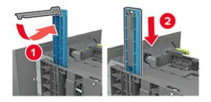
**d** Squeeze, and then slide the length guide to the correct position for the size of the paper being loaded.
