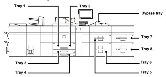
The setting orientation varies for the print side of paper, depending on the tray used. Place with the print side facing the direction indicated below.
