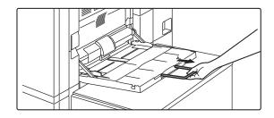
When loading paper larger than 8-1/2" × 11"R or A4R, pull out the extension guide.
