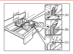
Adjust guide plates A and B by squeezing their lock levers and sliding them to match the longitudinal and transversal dimensions of the paper to be loaded.
