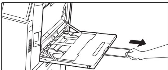
When loading paper larger than 8-1/2" x 11"R or A4R, pull out the extension guide. Pull the extension guide all the way out.
