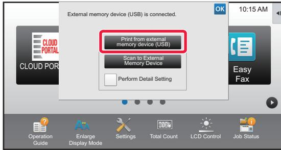
**When a screen for selecting the action appears, tap [Print from external memory device (USB)].**
