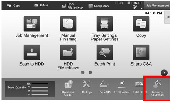
※When the machine is in process, machine cannot enter [Machine Adjustment] screen. If the [Machine Adjustment] is tapped the following messages appears with beep: Machine Adjustment is not available due to the job currently reserved/executed.
