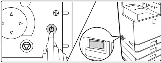
Press the [POWER] key (⏻) on the operation panel to turn off the panel power, and then switch the main power switch to the off position.
