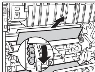
When the rotate knob is turned in the direction of the arrow, paper comes out for above.
