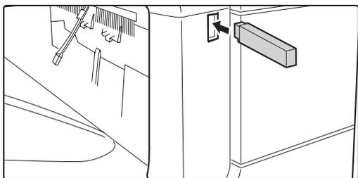
Connect the USB memory device to the machine.
