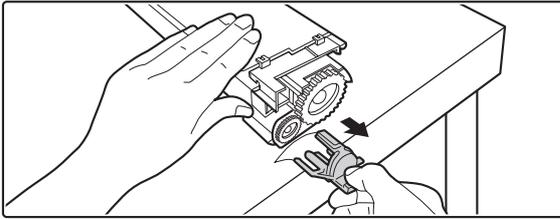
**Remove the protective material from the new toner cartridge.**
