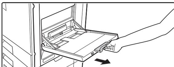
When loading paper larger than 8-1/2" x 11" or A4, be sure to pull the bypass tray extension all the way out. If the bypass tray extension is not pulled all the way out, the size of the loaded paper will not be correctly displayed.
