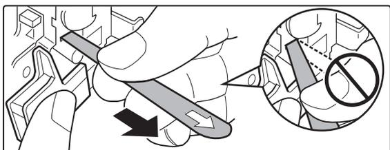
**Hold the developer cartridge with one hand and slowly remove the seal with the other hand.**
