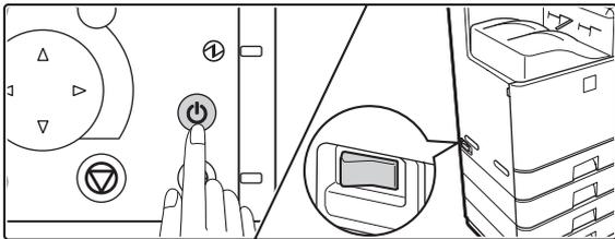
Press the [POWER] key (
