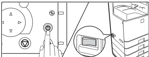
Press the [POWER] key (
