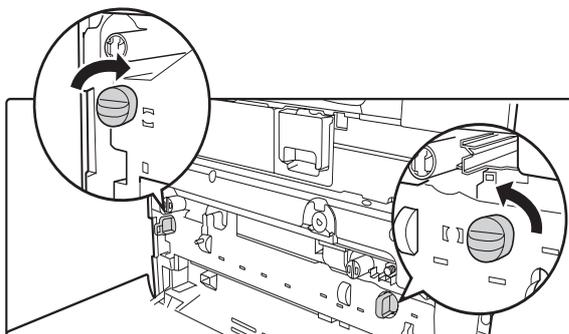
**Close the main charger cover and rotate the lock levers in the direction of the arrows to lock the cover.**
