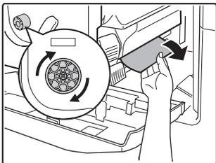
Turn roller rotating knob in the direction of the arrow to remove the misfed paper.
