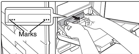
Remove the roller cover from the bypass tray.
