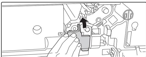
**Grasp the developer cartridge lock and replace it on the machine.**
