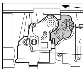
Drum cartridge alignment mark on machine
