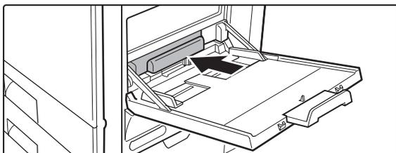
Attach the roller cover on the bypass tray.
