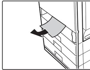
When a paper gets twisted to the roller, remove the tray and remove the misfed paper.
