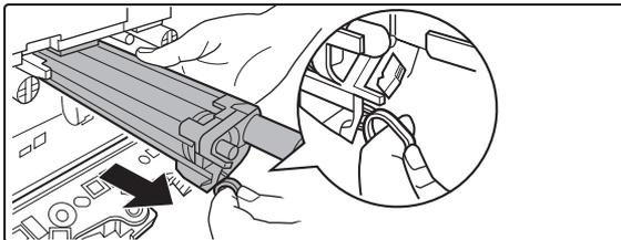
**Hold down the lever on the drum cartridge with your finger and pull the drum cartridge toward you.**
