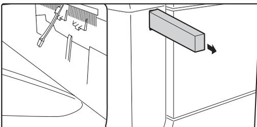
**Remove the USB memory device from the machine.**
