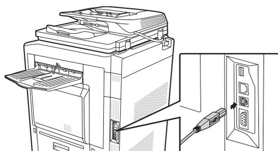
(3) **Connect the other end of the cable to the USB connector (A type) on your computer.**
