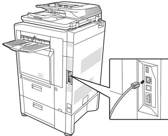
After connecting the machine to a network, be sure to configure the IP address and other network settings before installing the software. (The factory default setting for the IP address is to receive the IP address automatically when the machine is used in a DHCP environment.)
