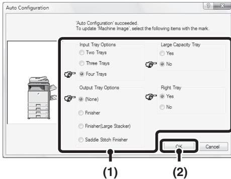
(1) Select the options that are installed on the machine.
