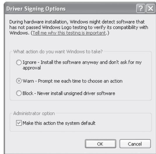
If [Block] is selected, the printer driver cannot be installed. Select [Warn] and install the printer driver again.
