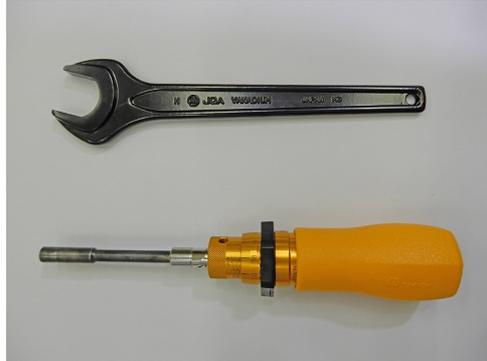
Make sure that the torque setting of the torque screwdriver is set to "180 cN·m" as shown in the figure below.
