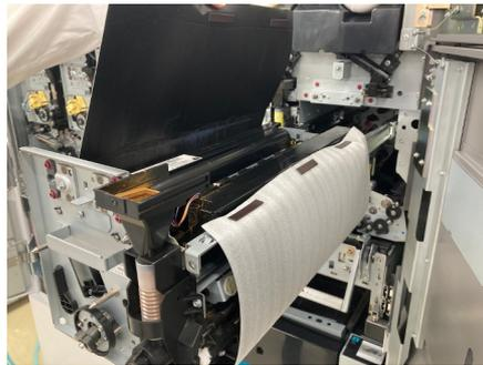
(2) Unlock the slide rails by pressing the lock, and house the marking module assembly inside the printer.
