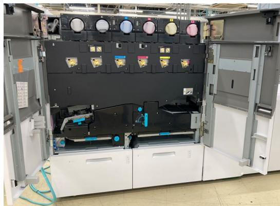
3. Rotate the handle of the transfer unit 2nd counterclockwise to unlock the unit. This sets the transfer unit 2nd to a lowered state.
