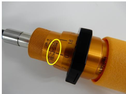
When using the torque screwdriver to tighten screws, be sure to turn the screwdriver until you hear the screwdriver click.
