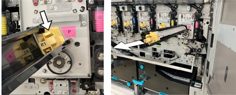
(4) Remove the corotron together with its protective cover, and place them on the upper lid of the storage box.
