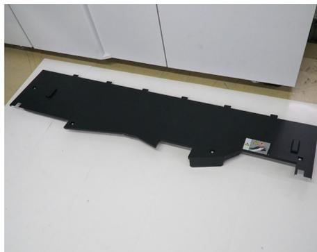
5. Remove the marking module cover.
