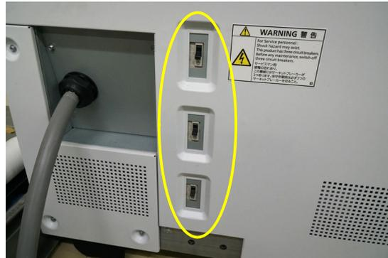
(2) Open the cover (right) of the printer output unit, turn the main power switch ON, and close the cover.
