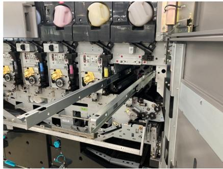
15. Open the toner cover on the side where it is to be replaced.
