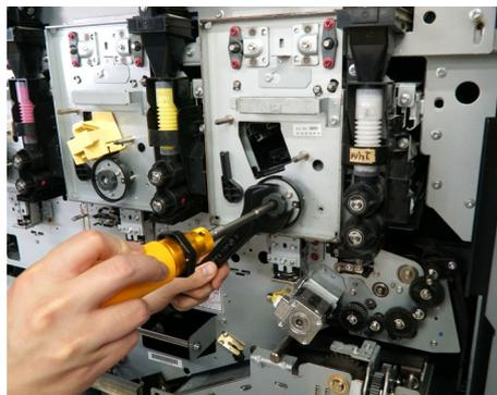
11. Draw out the marking module assembly and wind the drum light shielding sheet around the drum.
