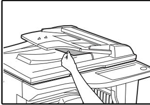
If the misfed original cannot be easily removed from the exit area, open the moveable part of the document feeder tray and remove the original.
