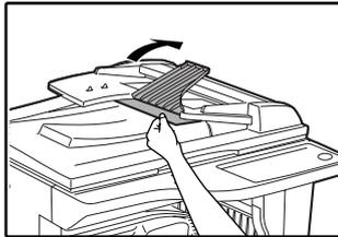
**2** Open and close the SPF to make the misfeed location indicator stop blinking.
