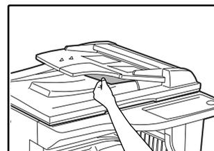
If a small original (5-1/2" x 8-1/2", etc.) is misfed, open the right side cover and remove the original. Close the right side cover.
