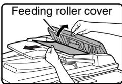
Open the feeding roller cover and gently remove the misfed original from the document feeder tray. Close the feeding roller cover.
