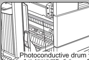
Do not touch or damage the photoconductive drum.
