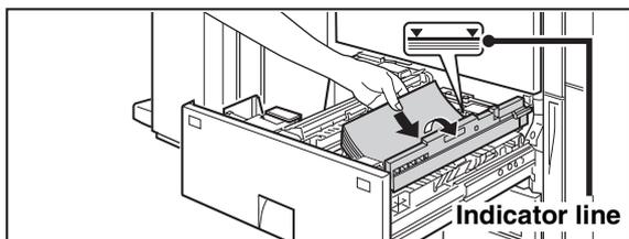
Raise the paper guide and load the paper with the print side face up. The stack must not be higher than the indicator line (maximum of 800 sheets).
