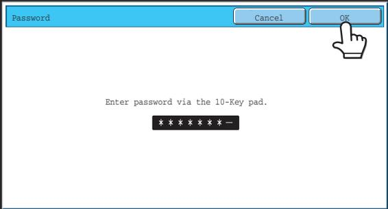
**Enter a password (5 to 8 digits) with the numeric keys and touch the [OK] key.**
