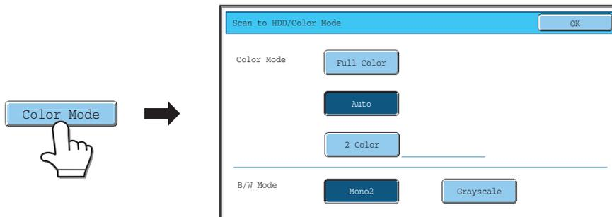
The following settings can be selected for the scanning color when the [COLOR START] key (●●●●) or the [BLACK & WHITE START] key (○●) is pressed.
