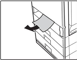
When a paper gets twisted to the roller, remove the tray and remove the misfeed paper.
