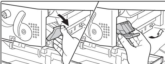
Lower the staple case release lever and remove the staple case.
