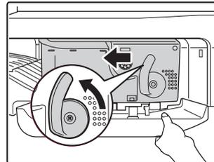
While pressing the lever over to the left, slide the finisher to the left until it stops.
