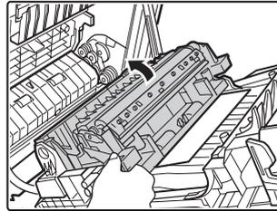
If the misfeed is not in the above location, grasp the handle on the secondary transfer roller unit, slowly open the unit, and remove the paper.
