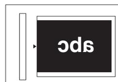
Align the right side of the original against the side of the document glass with the scale.
