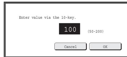
Press the numeric keys to enter any numeric value and then touch the [OK] key.
