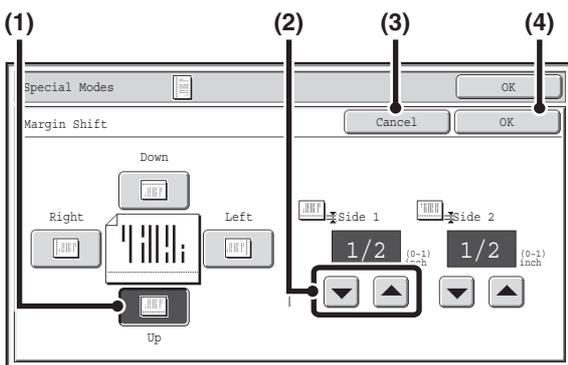
(1) If the initial state of a key in a screen is highlighted, the key is selected. To change the selection, touch one of the other keys to highlight that key.
