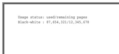
When page limits have been set in "Pages Limit Group List" in the system settings (administrator), the number of pages remaining will appear. (The remaining number of pages that the user can use in each mode (copy, scan, etc.) appears.) The amount of time that this screen appears can be changed using "Message Time Setting" in the system settings (administrator).
