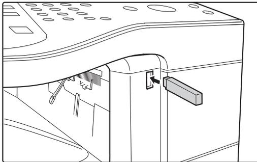
**Connect the USB memory to the USB connector (Type A) on the machine.**
