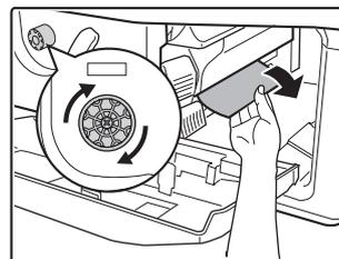
Turn roller rotating knob in the direction of the arrow to remove the misfeed paper.
