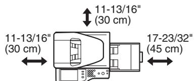
**CAUTION:****Do not install the machine in a location with poor air circulation.**
