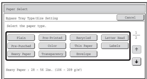
**Select the type of paper used in the bypass tray.**
