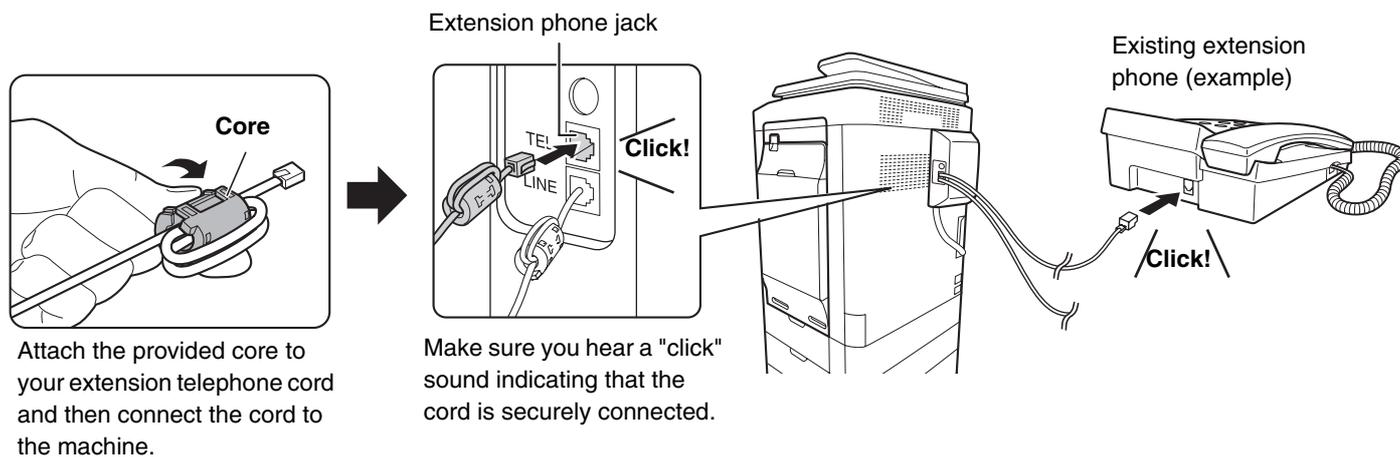
Attach the provided core to your extension telephone cord and then connect the cord to the machine.
