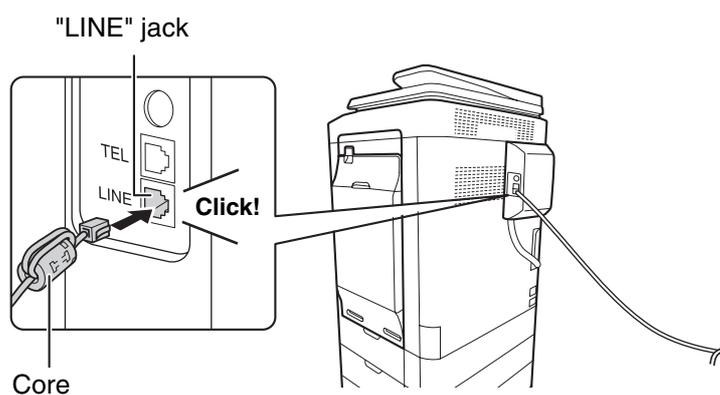
Insert the end of the cord with the core into the "LINE" jack.
