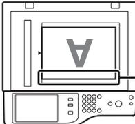
When using the staple sort function, place the original so that the top of the image is toward you.
