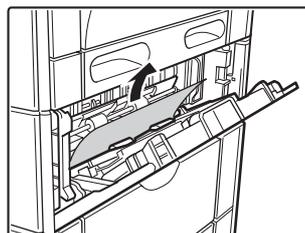
The misfeed may have occurred inside the machine. Check carefully and remove it.
