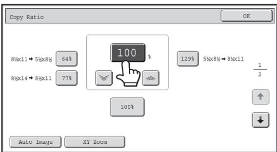
Touch a numeric value display key to directly enter a value with the numeric keys.
