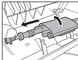
Remove the shaft rotating the roller cover upward and remove the shaft.
