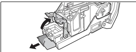
Raise the lever at the front end of the staple case and remove the jammed staple.
