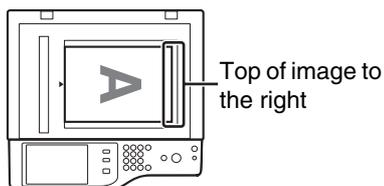
After placing the original, specify the original size.
