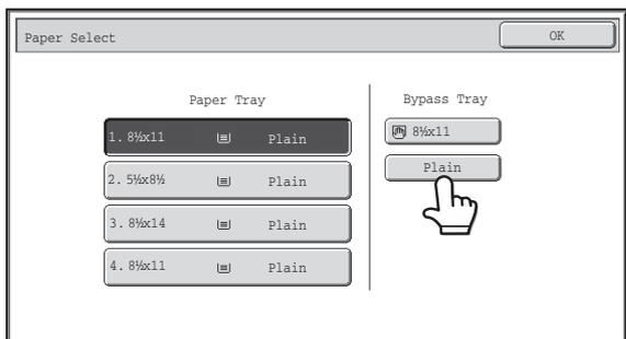
**Check the paper type setting for the bypass tray. If you need to change the setting, touch the paper type key.**
