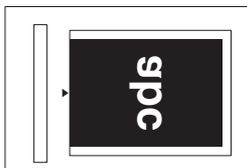
Align the top edge of the original against the side of the document glass with the scale.
