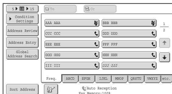
When destinations of other scan modes are stored in addition to fax destinations, an icon indicating the mode appears together with the name of the destination in each one-touch key.
