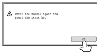
Touch the [OK] key, re-enter the destination with the numeric keys, and press the [BLACK & WHITE START] key.
