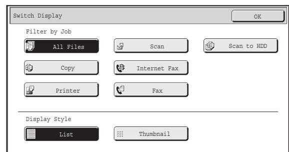
If you wish to display only the file keys of a specific job type, select the job type from the job type display at the top of the screen.
