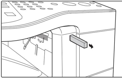
When "Sending data has been completed." appears in the touch panel, disconnect the USB memory.
