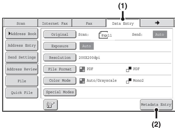
Switch to data entry mode and display the metadata set screen.
