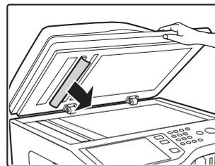
Open the automatic document feeder and remove the original.
