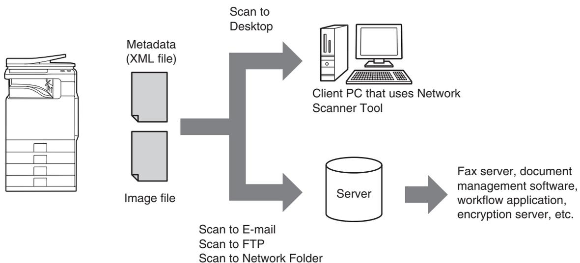
Using the application integration module kit, information on a generated image file can be entered at the touch panel and transmitted along with the image as an XML file.
