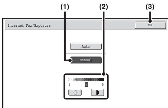
**(1) Touch the [Manual] key.****(2) Adjust the exposure with the
