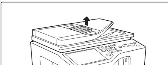
**After using the business card feeder, lift the feeder to remove it.**
