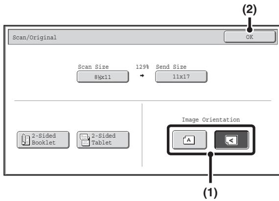
**Specify the orientation in which the original is placed.**
