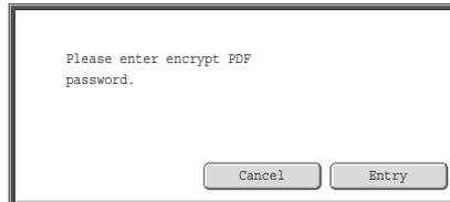
Touch the [Entry] key to open the keyboard screen, enter a password (maximum of 32 characters), and touch the [OK] key. The recipient must use the password entered here to open the encrypted PDF file.
