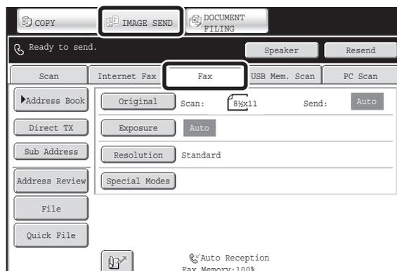
This screen only appears when the fax function and Internet fax function have been installed. The contents of the screen will vary depending on the devices that are installed.
