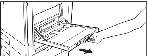
When loading paper larger than 8-1/2" x 11" or A4, be sure to pull out the bypass tray extension. Pull the bypass tray extension all the way out. If the bypass tray extension is not pulled all the way out, the size of the loaded paper will not be correctly displayed.
