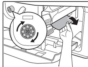
Turn roller rotating knob in the direction of the arrow to remove the misfeed paper.
