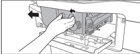
**3** Lower the staple case release lever and remove the staple case.
