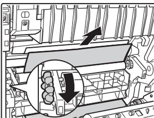
When the rotate knob is turned in the direction of the arrow, paper comes out for above.
