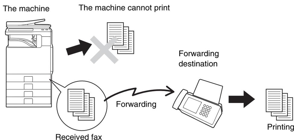
Forwarding of received faxes is executed in the system settings of the machine. Press the [SYSTEM SETTINGS] key on the operation panel to display the system setting menu screen in the touch panel. Select [Fax Data Receive/Forward] - [Fax Settings], and then touch the key that executes received fax forwarding.
