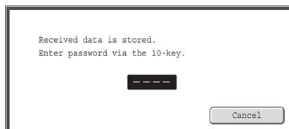
When the previously programmed 4-digit password is entered with the numeric keys, printing begins.
