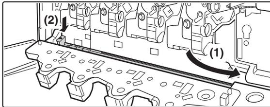
**Close the main charger cover and rotate the lock levers in the direction of the arrows to lock the cover.**
