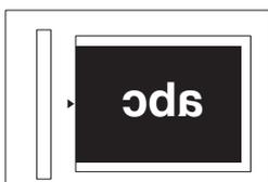
Align the right side of the original against the side of the document glass with the scale.
