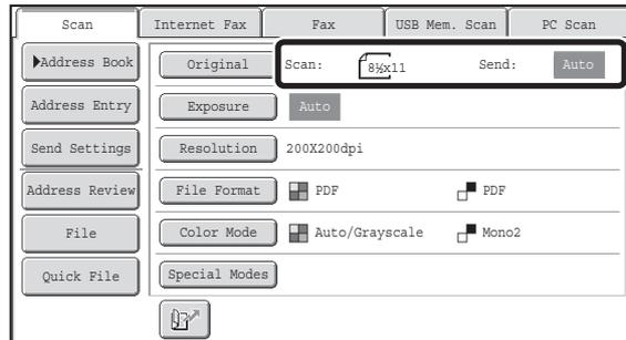
In the above screen, the scan size (the original size) is 8-1/2" x 11" (A4) and the send size is auto. For example, if the scan size is 8-1/2" x 11" (A4) and the send size is 5-1/2" x 8-1/2" (B5), the image will be reduced before transmission.
