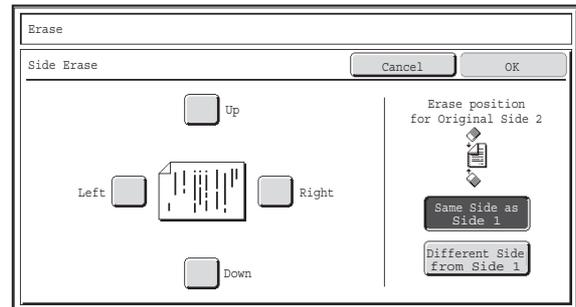
Touch the checkbox of the edge that you wish to erase and make sure that a checkmark () appears.
