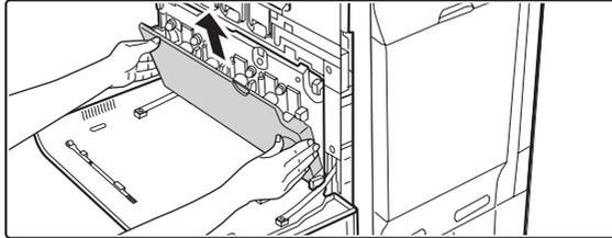
**Remove the cleaning tool for the writing unit from the front cover.**
