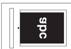
Align the top edge of the original against the side of the document glass with the scale.
