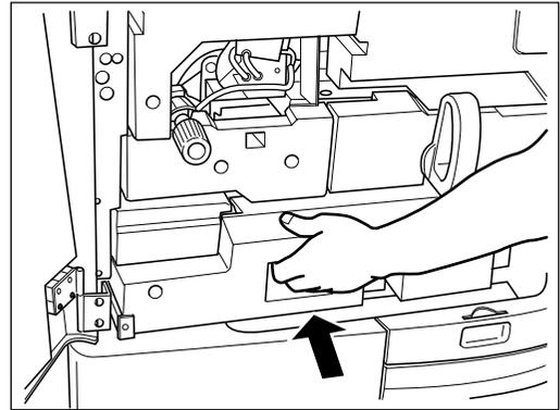
**18** Reinstall the large-capacity feeder.
