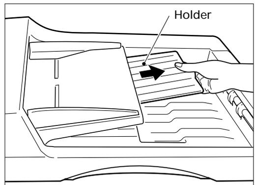
**Tip:** If you want to set more originals than the maximum number which can be set on the original feed tray at one time, you may add originals up to 3 times at the maximum. Press the **CONTINUE** key during the scanning. After scanning the loaded originals, place the next set of originals. Set the last pages of the originals first.
