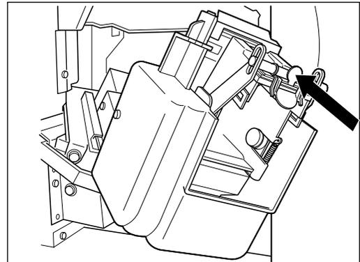
**9** Reinstall the stapler unit in its previous position.
