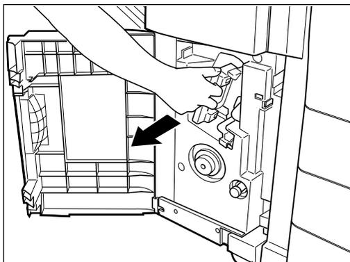
**3** Pull out the grip of the saddle stapler to the front and turn it 90 degrees to the right.
