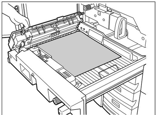
**14** Push the lock lever and open the transport unit cover.
