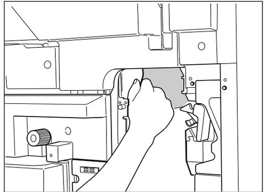
**10** Turn the knob counterclockwise and pull out the transport belt until it stops.
