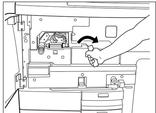
**14** Reinstall the large-capacity feeder and latch it.
