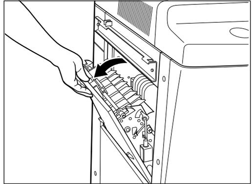
**3** If any paper is misfed in the exit side, remove it as shown.
