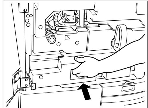
**18** Reinstall the large-capacity feeder.
