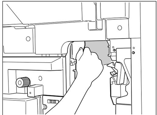
**10** Turn the knob in the direction shown and remove the paper if it comes out.
