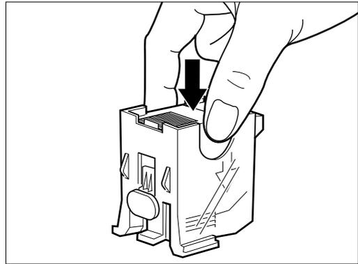
**7** Pulling straight up, remove the seal holding the staples.
