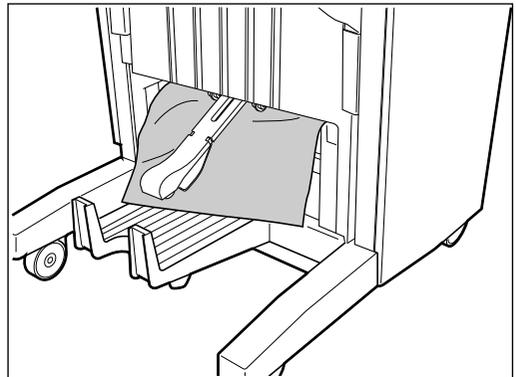
**7** If necessary, open the exit cover of the saddle stitcher and remove any misfed paper.
