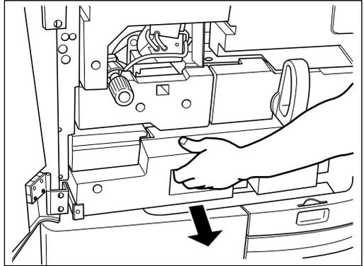
**12** Pull up the front lever of the automatic duplexer. If any paper is misfed inside, remove it as shown.
