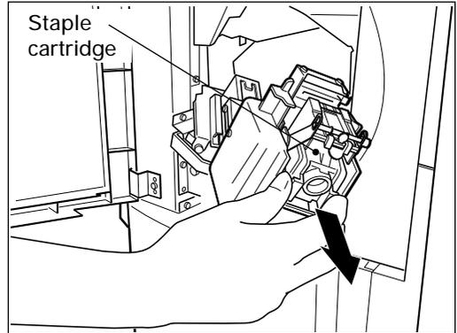
**6** Pull out the staple guide with the knob (2) while pushing the blue lever (1).
