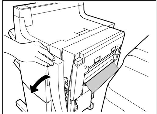
**2** Holding the black handle, slide out the case containing the paper bits, and dispose of them properly.
