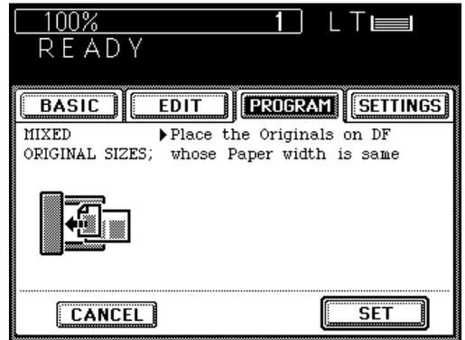
**4** Select the Automatic Paper Selection (APS) mode or Automatic Magnification Selection (AMS) mode. Then select the desired copy size, reproduction ratio, exposure and copy quantity as required.
