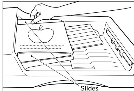
**Note:** Remove any paper clips or staples from originals before placing them on the original feed tray.
