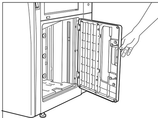
Note: If you want to add paper before the large-capacity feeder runs out of paper, press the TRAY DOWN
