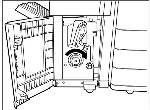
**6** Remove the paper misfed on the exit side of the saddle stitcher.
