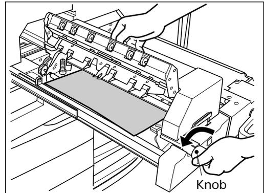
**13** Return the transport-belt unit until it comes to a stop and turn the knob clockwise to lock the lever.
