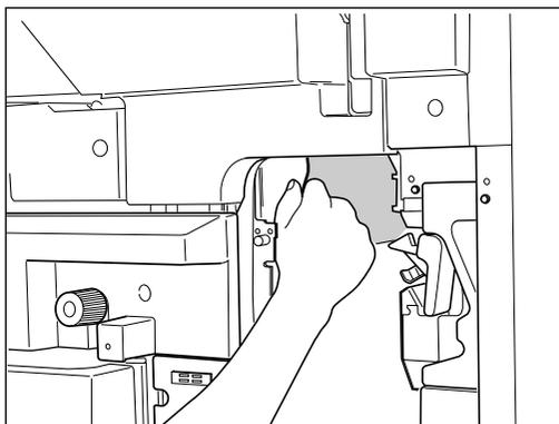
**4** Reinstall the large-capacity feeder and latch it.
