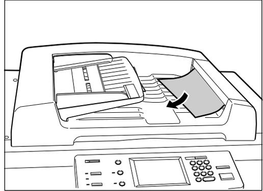
**2** Open the ADF exit cover and remove any foreign matter such as bits of paper, paper clips, etc.
