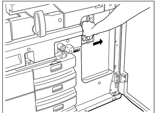
**8** Grip the lock lever to unlatch it and move the large-capacity feeder to the right slowly until it comes to a stop.
