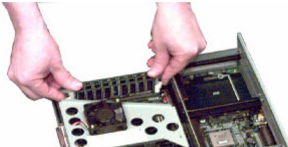
4. Replace the main board and secure it with the two screws.
