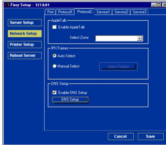
The Fiery supports the following Ethernet frame types for IPX/SPX: Ethernet 802.2, Ethernet 802.3, Ethernet II, and Ethernet SNAP. You can also allow the Fiery to select the frame type automatically.
