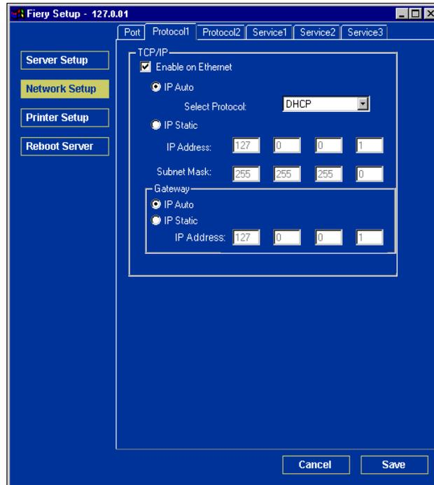
The Fiery requires a unique, valid IP address. You can set a static address or specify that the Fiery obtains the IP addresses automatically.
