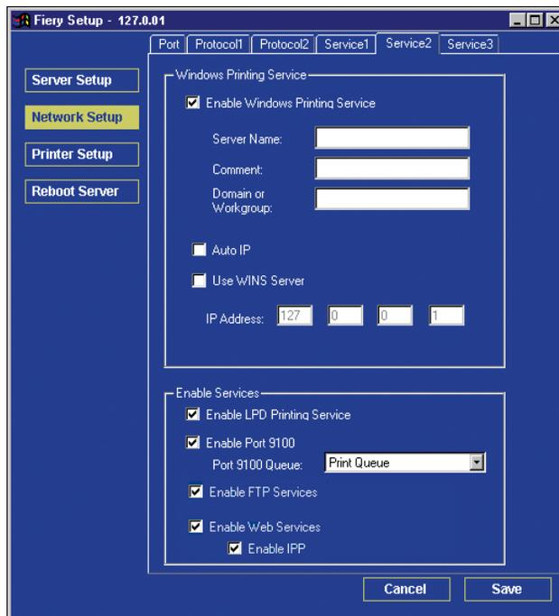
**Enable Windows Printing Service**—Select to enable SMB (Server Message Block), the file and printer sharing protocol built into Windows. Enabling SMB lists the Fiery on the network so that Windows clients can print to a particular print connection (Hold, Print, or Direct) on the Fiery without any other networking software. For information on setting up a Windows client for Windows printing, see the *User Software Installation Guide*.
