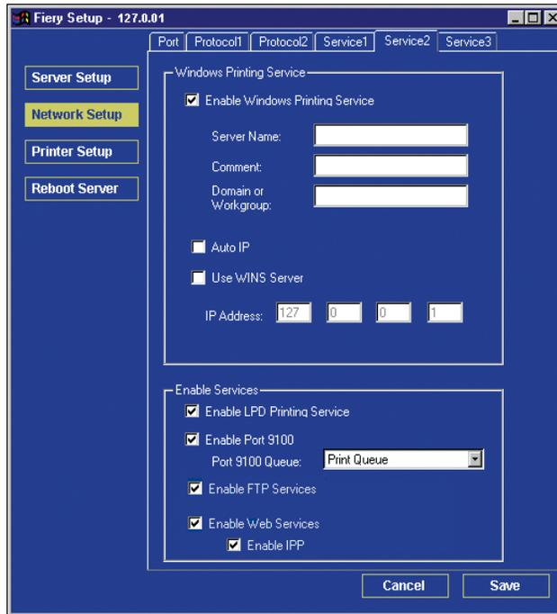
**Enable Port 9100**—Enables applications to open a TCP/IP socket to the Fiery at Port 9100 to download a print job.
