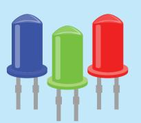
A pixel is a cluster of light emitting diodes (LEDs), which are tiny, electronic semiconductors that convert electrical energy into visible light.
