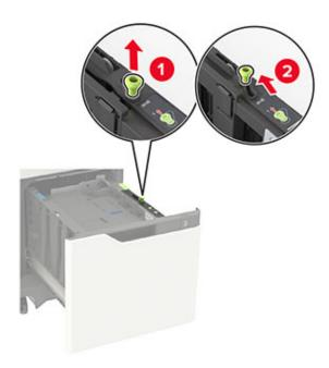
**b** If the A5 length guide is still attached, then remove it. If the guide is not attached, then proceed to <u>step</u> <u>d on page 25</u>.
