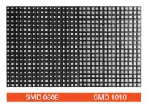
Compare the image of two LED modules with the same pixel pitch. The smaller SMD0808 diode has a larger ultra-black mask area visible between each diode compared to the SMD1010, resulting in a higher contrast. Naturally, there is a cost implication, but the resulting perceived image quality will be impacted by the size of the diode.
