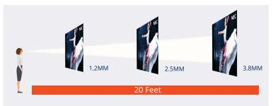
Pixel pitch is the distance from the center of a pixel to the center of any adjacent one. The smaller the pixel pitch, the higher the density and the clearer the image. Greater pixel density carries a higher price tag, so the best way to choose the right option is to consider the optimal viewing distance for the type of content whether its text, images or video; and its application - whether for company presentations or for digital signage.
