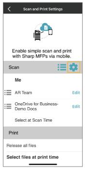
From the **Scan Settings** page, you can adjust default color mode, resolution (dpi), page size, file format, two-sided scan modes, blank page skip, compression, and compression ratio settings by choosing from the available options for the selected MFP.
